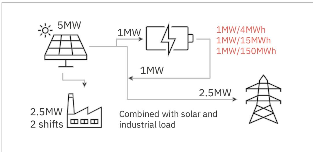
Figure 5 - Schematic overview of configuration with shared grid connection between industrial electric load and solar generation
