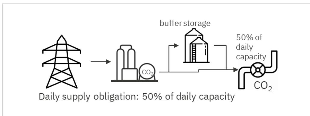
*Figure 6 – Schematic overview of configuration with merchant operation CO<sub>2</sub> production and daily delivery obligation*
