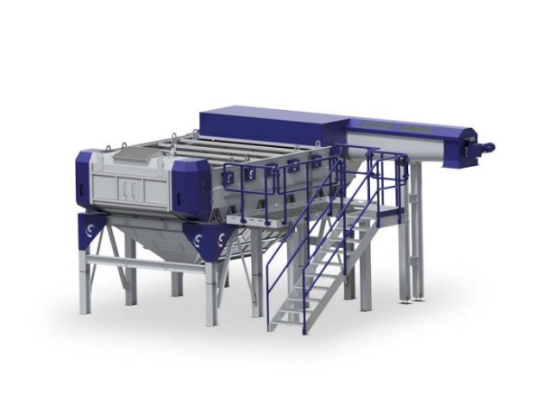
Figure 57. Float sink setup for plastic reprocessing (source Lindner Washtech ).
