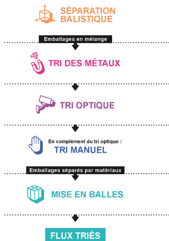
Figure 29. Typical sorting steps in French sorting installations (source: COTREP ).
