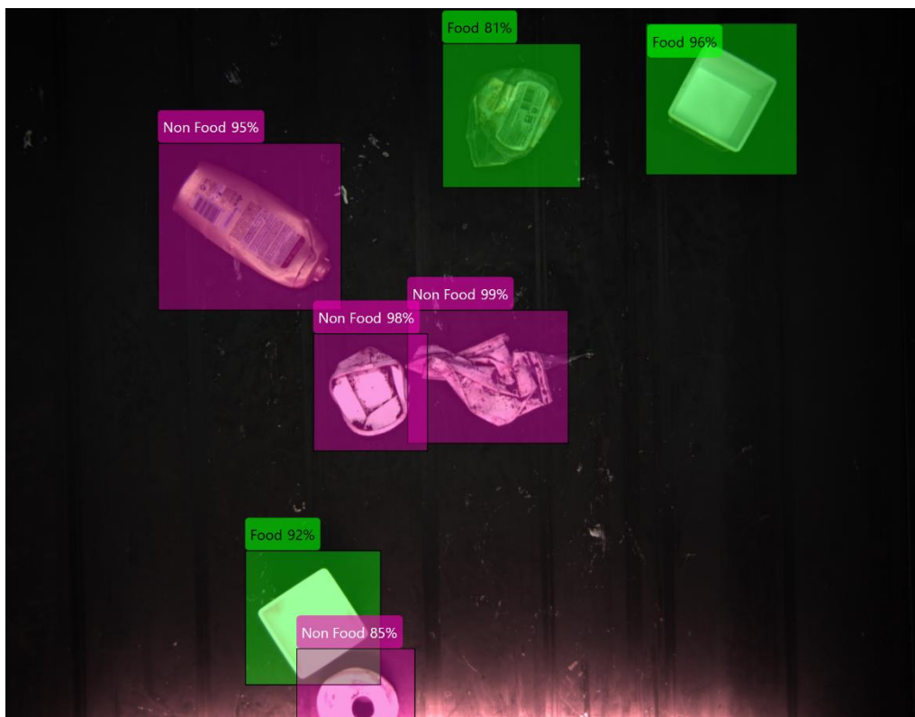
Figure 64. Vision and AI system that identifies food and non-food grade packaging
