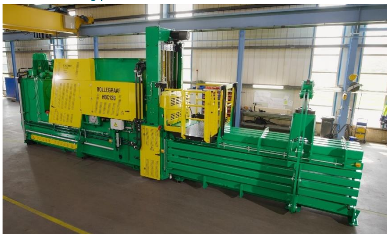
Figure 48. Typical baling press used in plastic packaging waste sorting (source: Bollegraaf ).
