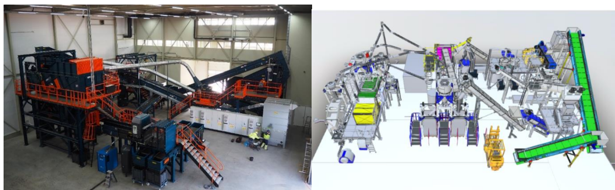
Figure 1. Sorting line (left) and schematic representation of recycling line (right) at NTCP.
